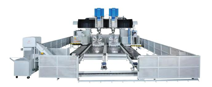
Johnford excels at putting customers' requirements and machining concept into realization. It has its own CNC department to program every machine, ensuring its reliability and functionality. For example, the 20-meter X-axis Portal Machining Center with a W-axis is a huge machine that only a few experienced manufacturers can make. Nevertheless, the company has already made over 5 of them.
