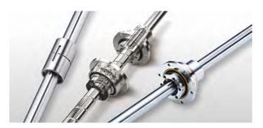
Some key technologies include its "Cross Roller Bearing" and "Cooling Nut System for Ball Screws". The "Cross Roller Bearing" are compact bearing with their rollers alternately crossed in a 90°v groove to each other between inner and outer rings.
